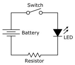
However, unlike breadboard diagrams, circuit diagrams only show *electrical* connections between components. They do not necessarily correspond to the *physical* layout of the components on a breadboard. For example, even though it looks different, this circuit diagram is identical to the previous one.
