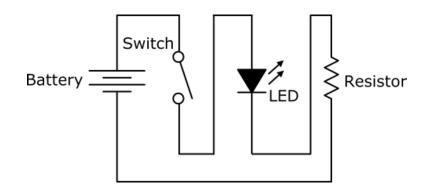
If you have a hard time understanding this, try using your figure to trace the "wire" (the black line) through the circuit, starting at the top of the battery. Notice how your finger still goes through each component in the same order, even though they have been physically rearranged.
