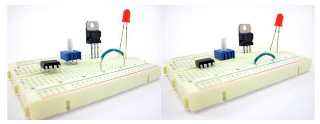
Note that some components, like LEDs, have very long leads that do not fit into the breadboard all the way. Other components, like pre-cut jumper wires, typically have leads cut to the right length, so they fit flush up against the breadboard.
