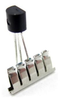
Some breadboards are actually made of transparent plastic, so you can see the clips inside.
