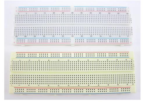
There may be small differences in how the buses are labeled from breadboard to breadboard. Some breadboards only have the colored lines and no plus (+) or minus (-) signs. Some breadboards have the positive buses on the left and the negative buses on the right, and on other breadboards, this is reversed. Regardless of how they are labeled and the left/right positions, the function of the buses remains the same.
