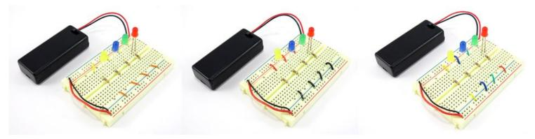
Remember the important part: the color of the wires does not affect how the circuit works! The three circuits in this image will all work exactly the same (the LEDs will light up when the battery pack is turned on) even though they have different color wires. If a breadboard diagram shows a blue wire and you use an orange wire instead, nothing will be wrong with your circuit.
