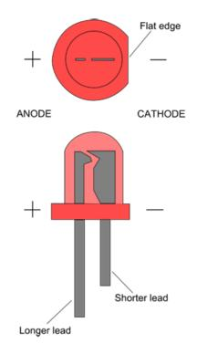
**Diodes** are like one-way valves that only let electricity flow in one direction. They are usually small cylinders marked with a band or stripe on one end (this is the direction electricity can flow toward).
