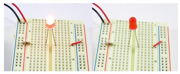
Do you see the problem yet? In the photo on the left, the red jumper wire goes to the positive (+) bus. In the photo on the right, it goes to the negative (-) bus. According to the breadboard diagram from the previous section (#row-numbers), it should go to the positive (+) bus. Remember that "positive" and "negative" can also be referred to as "power" and "ground." See the section on buses (#lines) if you need a reminder.
