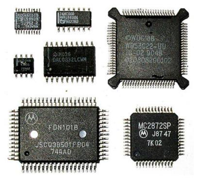
Many electronic components are available in both through-hole and surface mount packages. For example, the LM3914 (http://www.avantiink.com/click.php?
