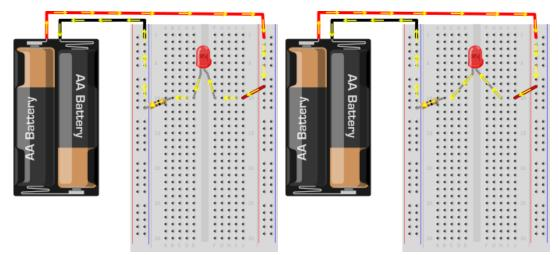
However, you can also completely rearrange the components on the breadboard. As long as the circuit is *electrically* equivalent, it will still work. Even though this circuit "looks different" than the previous two because the components have been rearranged, electricity still follows an equivalent path through the LED and the resistor.
