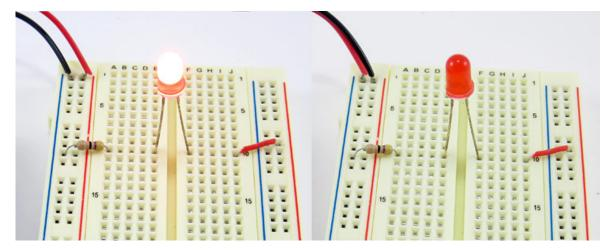
This time, the battery pack leads are reversed. The red lead is connected to the negative (-) bus and the black lead is connected to the positive (+) bus. Remember that unlike with jumper wires (#jumper-wires), the colors of battery pack leads *do* matter. Red is used for positive and black is used for negative.
