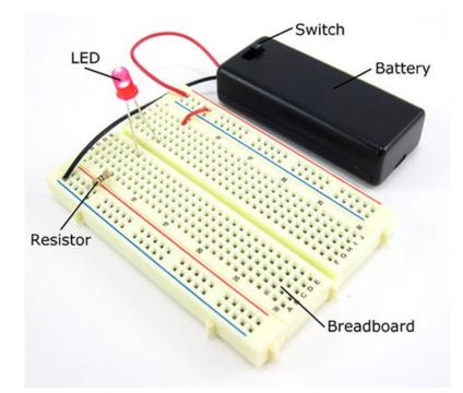
The connections are not permanent, so it is easy to *remove* a component if you make a mistake, or just start over and do a new project. This makes breadboards great for beginners who are new to electronics. You can use breadboards to make all sorts of fun electronics projects, from different types of robots or an electronic drum set, to an electronic rain detector to help conserve water in a garden, just to name a few.
