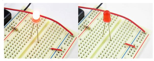
Do you see the problem yet? In the circuit on the left, the red jumper wire goes from the positive bus to hole J10, which matches the breadboard diagram. In the circuit on the right, it goes from the positive bus to hole J9. Remember from the section on how the holes are connected (#holes) that holes in different rows are not electrically connected to each other. So, with the jumper wire in row 9 and the LED in row 10, there is no way for electricity to flow to the LED.
